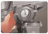
Insert the convertible top release tool (from the glove box) or your ignition key and turn it to activate the emergency release. To remove the cargo cover, see your Owner Manual for full details.
